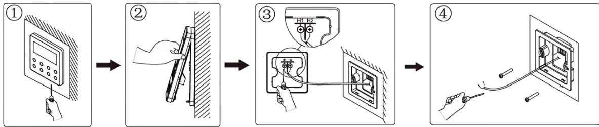
Figure 2-5-3 Removal of wired controller
