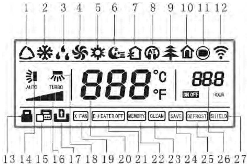
Figure 2-3-2 LCD display of wired controller
